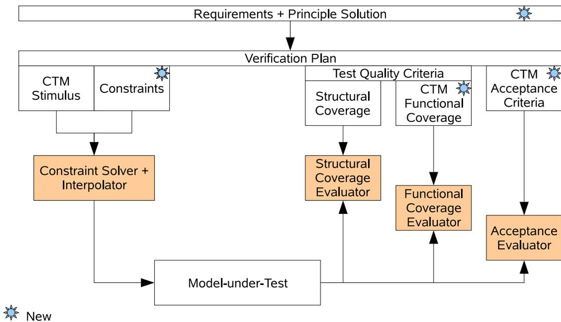
Figure 3: Verification Plan for Systematic Testing
