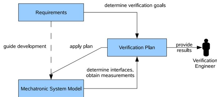
Figure 1: Verification Plan, Requirements and Mechatronic Model
