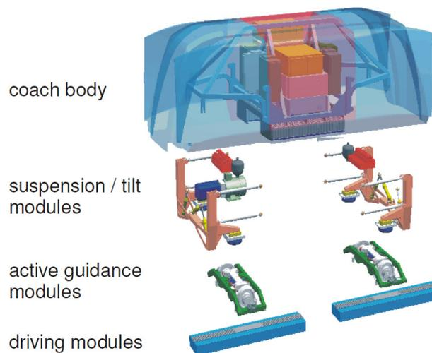
Figure 2: Modules of the RailCab Shuttle
